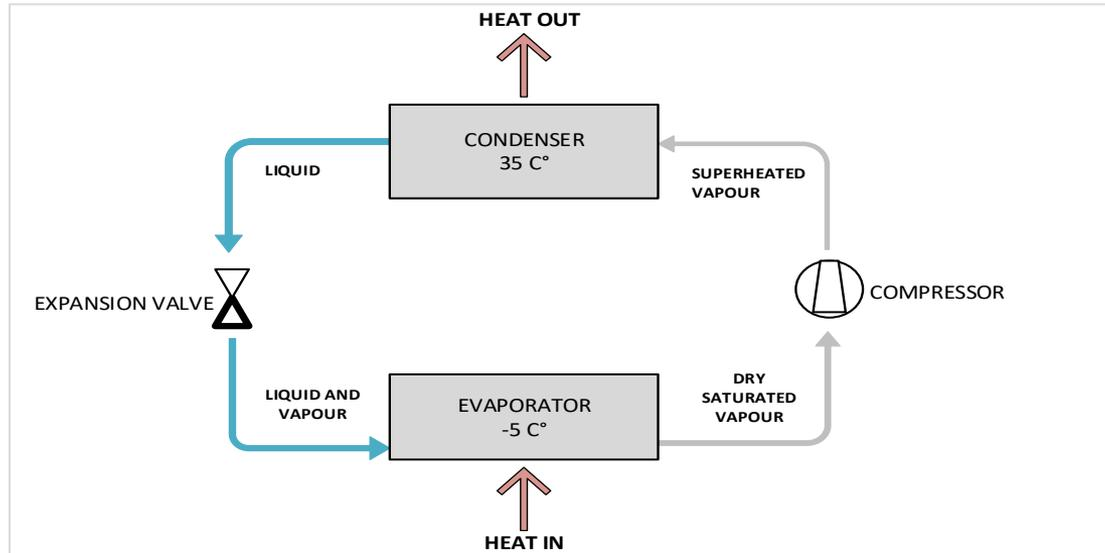
Most heat pumps use a mechanical vapour compression cycle with the compressor driven by an electric motor. Standard vapour compression heat pumps work by alternately evaporating and condensing a refrigerant. The main components are shown in the figure above and include: an evaporator, a compressor, a condenser, an expansion valve and a refrigerant such as R410A. Standard heat pumps are able to efficiently provide water flow temperatures of up to 55°C.
